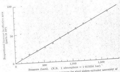
Fig. 1. Dependence of effective area on pressure for steel piston-cylinder assembly of
